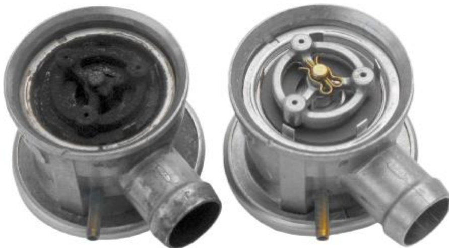
Cut-off secondary air valve left: stuck by deposits – right: in new condition
