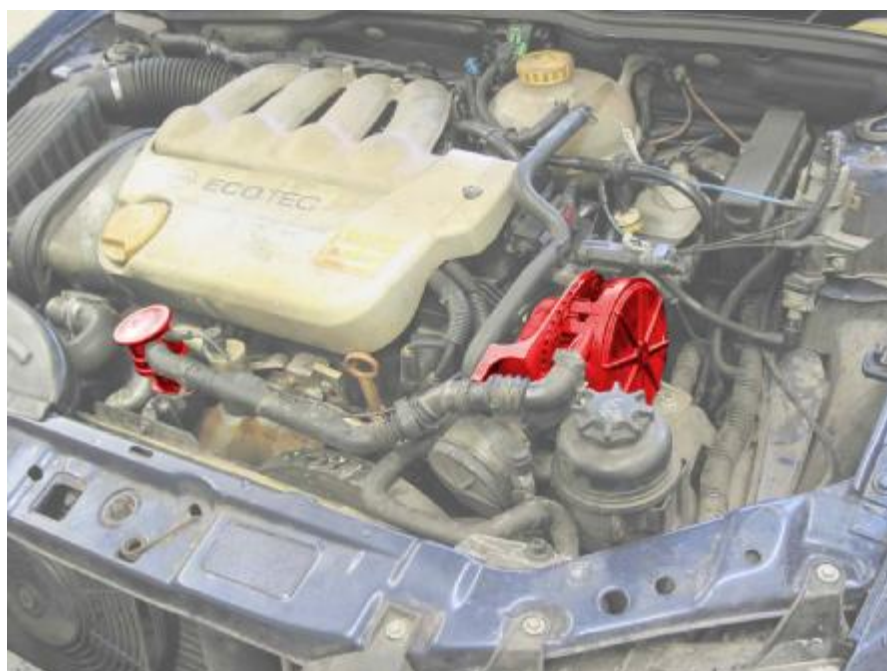
Secondary-air valve and secondary air pump in Opel Tigua (highlighted)
