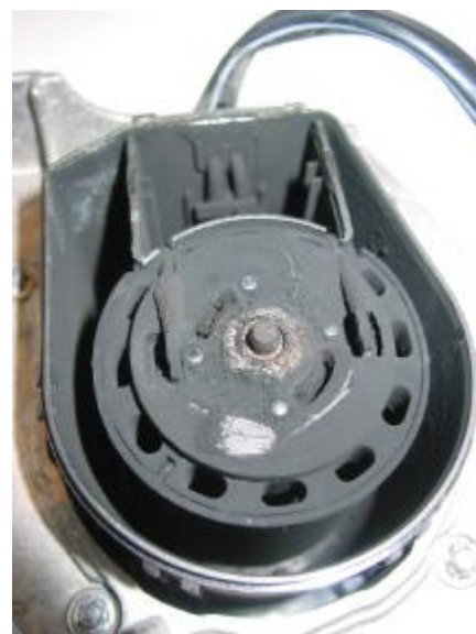
Secondary "soot" pump? The interior of a secondary air pump should not look like this.
