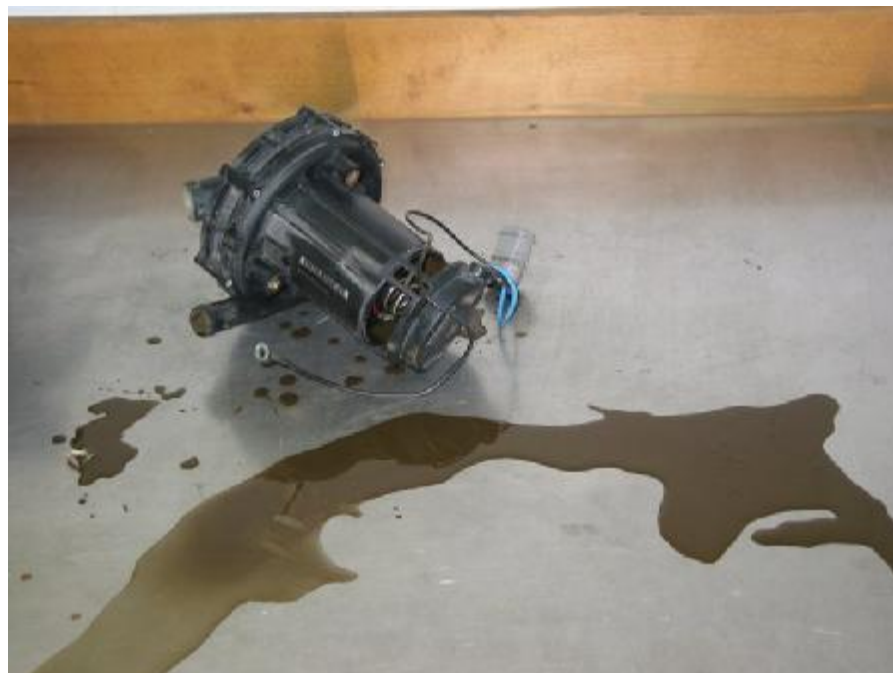
Secondary "water" pump? From time to time, we receive secondary air pumps as warranty returns which are still filled with aggressive exhaust-gas condensate. Since the non-return valve is intended to prevent this, it must be defective.
